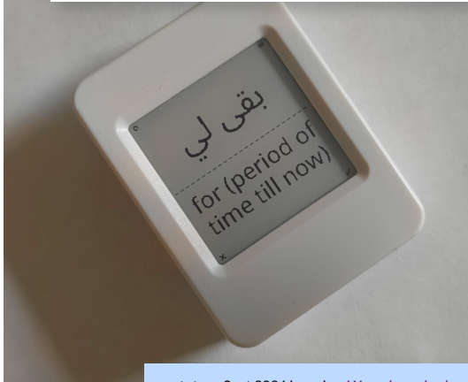
prototype Sept 2026 based on Waveshare dev board
